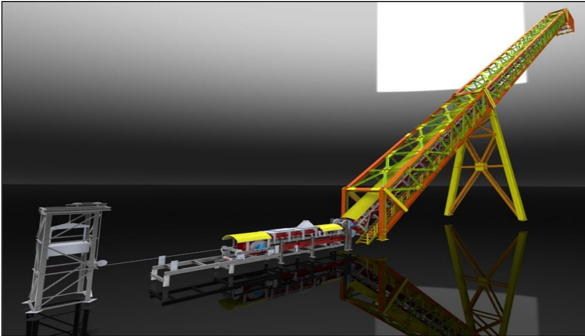
Direct reduced iron transfer sidewall belt engineering model- Pasargad Steel (iron smelting) Co.
